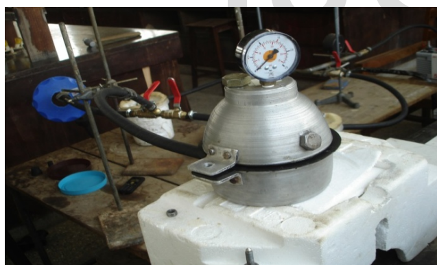
Fig. 1: PV cell with pressure gauge fitted on the feed chamber.
